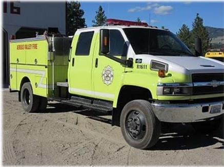
*Rescue vehicle* – This 2005 Kodiak is a replacement vehicle for our current 1-ton rescue vehicle as well as being capable of fighting both wildland and structure fires with its 4x4 drive and 500 gallons of water. We added a service box purchased from FD 4 to support its multi-function role.
